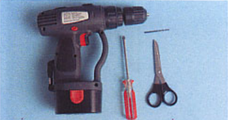
1. Fitting tools required include star point screwdriver, scissors, drill & Ø2.5mm drill bit
